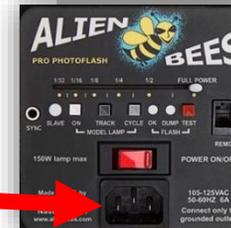
3. Plug power cable into back of flash
