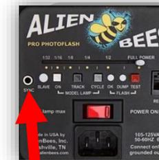
4. SYNC cable from wired transmitter on camera will plug into SYNC port on back of flash
